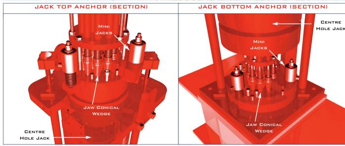
Fagioli's Cable net Lifting & Tensioning System jacks are equipped, both at top and bottom anchor, with secondary hydraulic systems named MINI JACKS which are incorporated in the gripping mechanism to override their automatic operation. This secondary hydraulic system allows the jacks to be opened without lifting during resetting and also allows the cable to pass through the lower grips when lowering.
