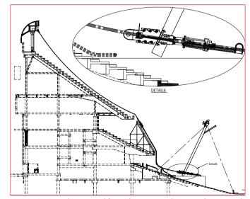
STAGE 6 - Strands removed from the pattern plates one by one and threaded on to jacks / strands fitted on strand guides
