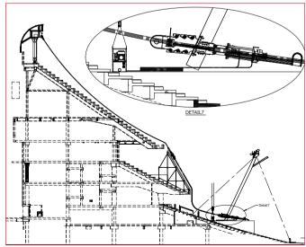
STAGE 7 - Power pack units installed / electrical & hydraulic equipment installed on jacks and connected to PPUs
