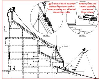
STAGE 4 - Upper anchor beam assembly, lifted with strands and pattern plates trailing
