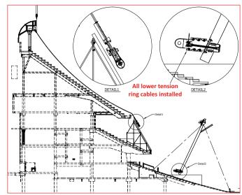
STAGE 2 - Lower anchor beam assembly installed on Lower Radial Cables / Lower Radial Cables installed on compression ring
