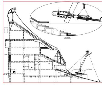
STAGE 5 - Jacks and jack support beam assemblies installed on bottom of the flying columns
