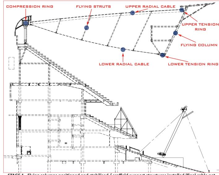
STAGE 1 - Flying columns positioned and stabilised / scaffold support structures installed (final cable net position shown for clarity)
