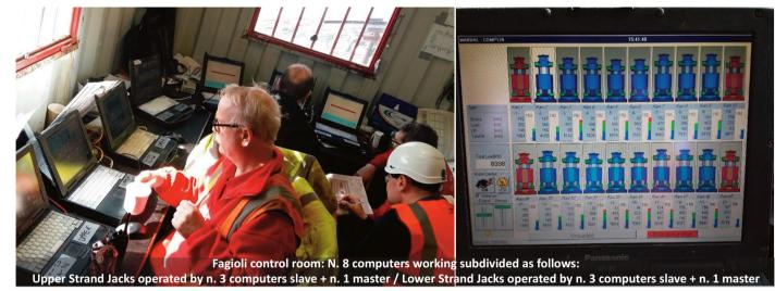
In the combined computer control/manual system configuration, the term "manual control" means that the operation can be performed by the lead supervisor controlling the computer assisted by a skilled operator that visually observes each and every jack in function and reports by radio the status of the hydraulic piston stroke at an axis to the lead operator.
